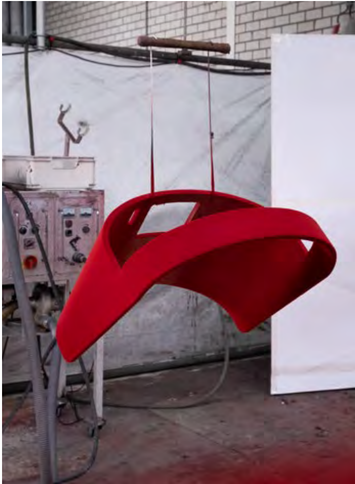
Applying the flock coating at Flock Techniek in Geldrop Photography: Chiara Catalini
