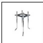
S.2840 PLANTED ROOT for CYLINDRICAL POLE S.2846, S.2848 h = 550 mm and bolts in galvanized steel with M16 threads. Suggested reinforced concrete footstall dimension: A = 0.7 m B = 1 m
