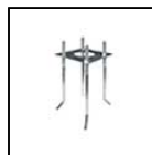
S.2849 PLANTED ROOT for CYLINDRICAL POLE S.2801, S.2813, S.2843, S.2845 C= 200mm, D=200mm E=Ø80mm, h=460mm, h1=90mm and bolts in galvanized steel with M16 threads. Suggested reinforced concrete footstall dimension **: A = 0.7 m B = 0.7 m **Footstall dimension can be calculated according to your country norms and ground properties.
