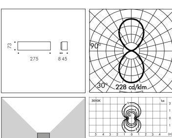
\*Photometric measured using WHITE LED 3000K
