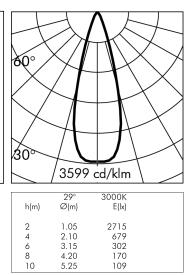
\*Photometric measured using WHITE LED 3000K
