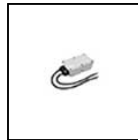
S.2492 Virtual Midnight Interface Device IP20 Compact control IP20 module for automatic power reduction / brightness reduction for night-time. The device has an integrated bus supply (20mA) for up to 7 DALI luminaires. Possibility to extend up to max. 64 luminaires through the DALI Expander (S.2494). 2 operating modes are supported: - Operating mode B1: power reduction through mains phase or control phase; - Operating mode B2: power reduction using virtual midnight calculation. All necessary settings can be made using rotary and slide switches. The device must be located before the DALI luminaire inside an electrical cabinet / waterbox / junction box.
