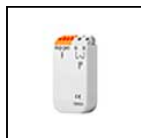
S.2495 DALI2 RELAY SWITCH for ON-OFF (NOT DIMMABLE) 230V LUMINAIRES Allows to make a remote control of ON-OFF not dimmable 230V luminaires via DALI2 protocol. IP20 Max nominal load 1000VA Max switching current 8A Max inrush current 80A Dimensions 32,5mm x 15mm x 58,5mm NB: the Luminaire can be controlled remotely in ON-OFF mode only and not in dimmed mode. The total quantity of the Inrush currents of the luminaires/fixtures that you want to connect to the DALI2 RELAY SWITCH, must not exceed the maximum value of 80A.
