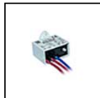
S.2499 SURGE PROTECTION DEVICE 10kV CLASS II Compatible with all lighting fixtures and electronic ballast accessories classified under electrical Protection Class II Rated voltage 230-277V SPD type 2+3 Max Surge Protection 10kV IP67 EACH FIXTURE MUST BE CONNECTED TO ONE SINGLE SURGE PROTECTION DEVICE AT A DISTANCE OF NO MORE THAN 10m AWAY.
