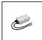
S.2496 DALI2 RELAY SWITCH for ON-OFF (NOT DIMMABLE) 230V LUMINAIRES Allows to make a remote control of ON-OFF not dimmable 230V luminaires via DALI2 protocol. IP67 Max nominal load 1000VA Max switching current 8A Max inrush current 80A Dimensions 175,5mm x 86,5mm x 43mm NB: the Luminaire can be controlled remotely in ON-OFF mode only and not in dimmed mode. The total quantity of the Inrush currents of the luminaires/fixtures that you want to connect to the DALI2 RELAY SWITCH, must not exceed the maximum value of 80A.
