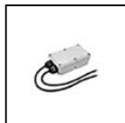
S.2496 DALI2 RELAY SWITCH for ON-OFF (NOT DIMMABLE) 230V LUMINAIRES Allows to make a remote control of ON-OFF not dimmable 230V luminaires via DALI2 protocol. IP67 Max nominal load 1000VA Max switching current 8A Max inrush current 80A Dimensions 175,5mm x 86,5mm x 43mm NB: the Luminaire can be controlled remotely in ON-OFF mode only and not in dimmed mode. The total quantity of the Inrush currents of the luminaires/fixtures that you want to connect to the DALI2 RELAY SWITCH, must not exceed the maximum value of 80A.
