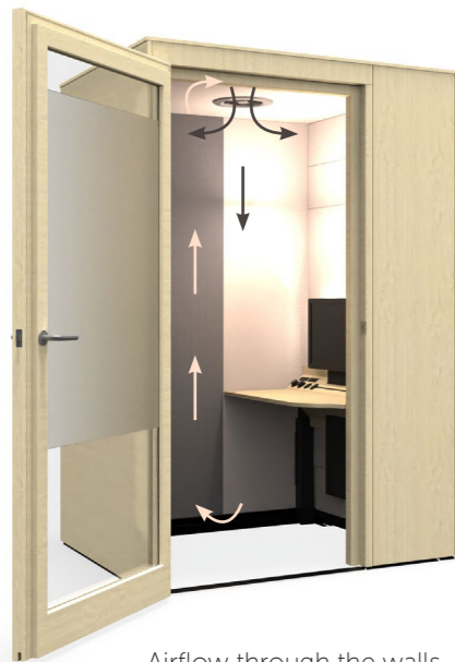
Airflow through the walls
