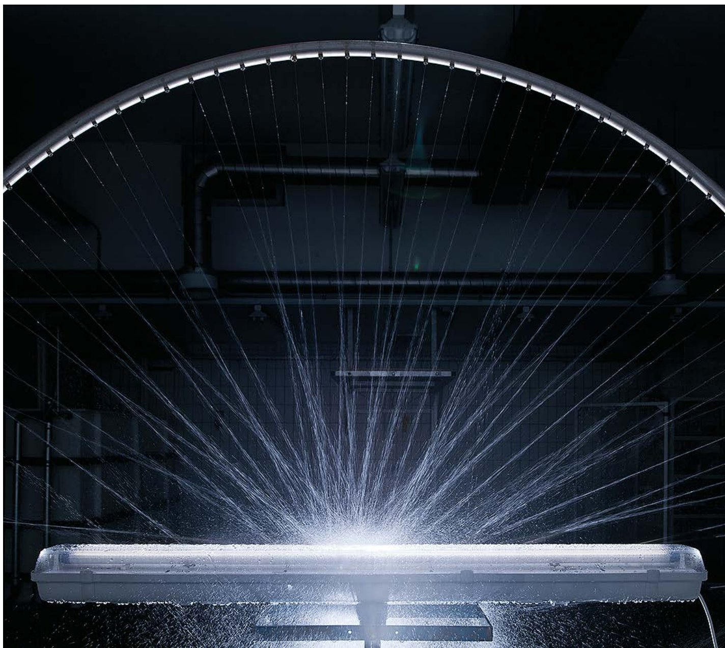
The water resistance of Zumtobel luminaires is tested under extreme conditions to maintain outstanding levels of reliability.
