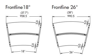
The Frontline end panel has a 0.16" (4 mm) flat front edge of solid wood. The distance between the front edge of the end panel and the front edge of the shelf is 0.02" (5 mm).
