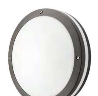
Attractive, round luminaire with direct and indirect light that can be mounted to both walls and ceilings, and both indoors and outdoors. Made of die-cast powder-coated aluminium. Flat diffuser with indirect light made of UV-stabilised opal polycarbonate. Two inputs/outputs for cables, option of both visible and concealed cabling, and loopable quick clips. Design: Hallvard Jakobsen
