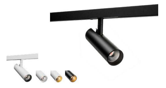
Slim, precise spotlight for Zip 230V rail system. The luminaire has a minimalistic, exclusive look. Made of powder-coated, die-cast aluminium and available in black or white finish. The retracted light source causes minimal glare and can be dimmed with trailing edge dimmer. Tube Micro Black comes with black and gold bezel ring, Tube Micro Whire comes with black, white and gold bezel ring.
