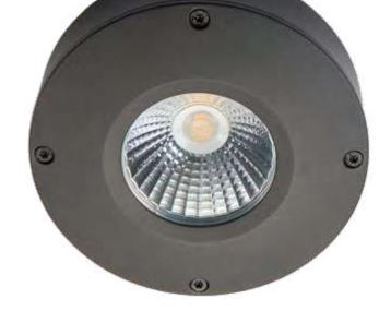
Good little LED luminaire for walls and ceiling. For both outdoor and indoor use. Well integrated LED chip, dimmable via phase-dimming. Made of die-cast powder-coated aluminium, powder coating and 10-year corrosion warranty, glass diffuser. 33mm in total height, Cl II means that it can be mounted without earthing, direct 230 V with loopable quick clips.
