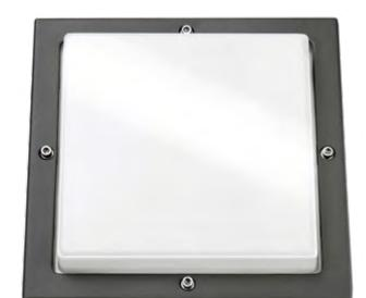
Attractive, square LED wall luminaire that can be installed both indoors and outdoors. Made of die-cast powder-coated aluminium. Diffuser made of UV-stabilised opalescent polycarbonate, two inputs/outputs for cables, option of both visible and hidden cabling, and loopable quick clips.
