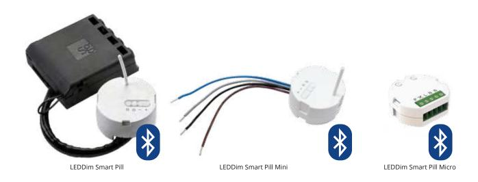
LEDDim Smart Pill is a dimmer that can be installed in a recessed ceiling, a wall box or similar in order to control one or more fittings. The dimmer is controlled via app using Bluetooth (BLE), Smart Switch or using a push switch.
