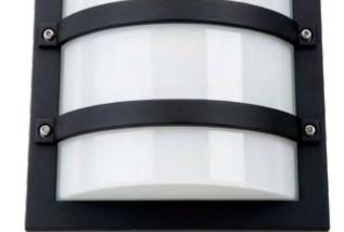
Square wall luminaire with extra protection of diffuser. Made of die-cast powder-coated aluminium. Diffuser made of UV-stabilised opal polycarbonate. Two inputs/outputs for cables, option of both visible and concealed cabling, and loopable quick clips. Design: Hallvard Jakobsen
