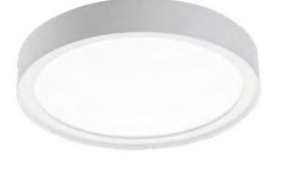
Energy efficient surface-mounted LED fixtures with a slim profile ensuring a modern look. Square and round available in multiple sizes and lumens. Opal-prismatic diffuser provides a glare-free light. Dimmable using a DALI or trailing edge dimmer. Simple installation with quick connections between fixture and back plate that can be screwed straight onto all known ceiling boxes. Visible cabling also possible.
