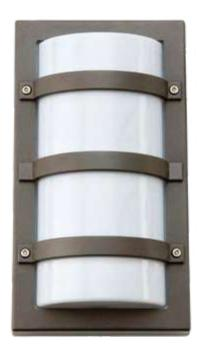
Square wall luminaire for extra protection of diffuser. Made of die-cast powder-coated aluminium. Diffuser made of UV-stabilised opal polycarbonate. Two inputs/outputs for cables, option of both visible and concealed cabling, and loopable quick clips. Corrosion-proof with 10-year warranty, IP65 and vandal-resistant rating IK10.
