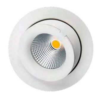
Attractive downlight for indoor and outdoor use, particularly well suited to sloping ceilings and effect lighting via the unique 40-degree trunk tip. Well integrated LED chip and associated dimmable driver. Made of die-cast aluminiuim in powder coated or brushed steel finish. Glass diffuser. 42-degree beam angle. Low recessed downlight.
