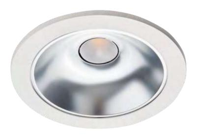
Flush-mounted LED downlight. Made of fire-resistant polycarbonate. SDCM 2. L90/B10>100,000, Supplied with 3000K/4000K LED. Complete with driver and quick connection between driver and downlight for super quick and easy mounting. Can be mounted to ceiling panels with a thickness of 1–50 mm. The luminaire comes complete with ceiling ring made of die-cast aluminium. Matt reflector.
