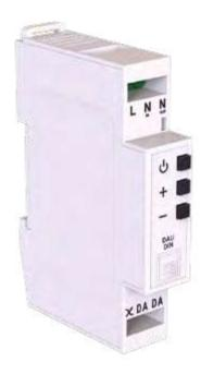
Implement all phase control dimmable light sources using DALI. Convert a DALI signal into phase control dimming. Can be used anywhere you wanted a phase control dimmable fixture in a DALI installation. You can connect multiple phase control dimmable fixtures to one shared DALI address, enabling a simpler installation with fewer DALI addresses. Save time and money compared with a full DALI installation. Installed on DIN rail.
