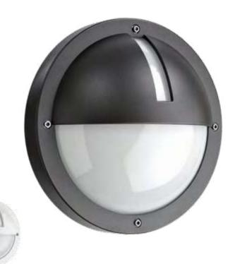
Attractive, round wall luminaire with half-diffuser and slit that can be installed both indoors and outdoors. Made of diecast powder-coated aluminium. Diffuser made of UV-stabilised opal polycarbonate.
