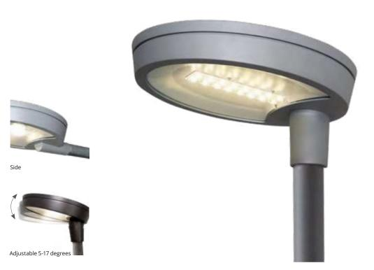
Light for mounting on mast, IP66-rated. Luminaire body made of die-cast aluminium, powder-coated in black or grey. Reflector made of aluminium, powder-coated white. Optics are particularly well suited to giving a direct light distribution due to the tempered glass front. Complete with LED driver for operation of LED light sources mounted to component rail pre-mounted with six-metre connection cable. Lamp head prepared for mounting on 60 mm mast. Design: Christian Hvidt
