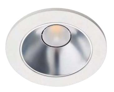
Flush-mounted LED downlight. Made of fire-resistant polycarbonate. Complete with driver and quick connection between driver and downlight for super quick and easy mounting. Can be mounted to ceiling panels with a thickness of 1–50 mm. The luminaire comes complete with ceiling ring made of die-cast aluminium. Matt reflector.
