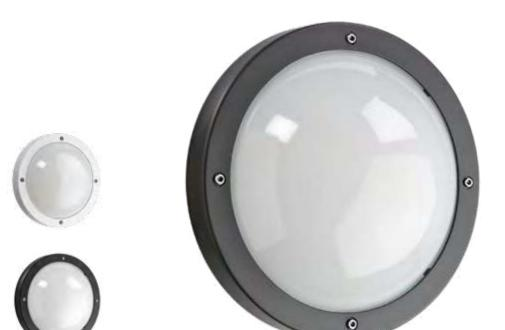
Attractive, round wall luminaire that can be installed both indoors and outdoors. Made of die-cast powder-coated aluminium. Diffuser made of UV-stabilised opal polycarbonate. Two inputs/outputs for cables, option of both visible and concealed cabling, and loopable quick clips. Corrosion-proof with 10-year warranty, IP65 and vandal-resistant rating IK10. Variants with integrated sensor or Twilight relay. Design: Hallvard Jakobsen
