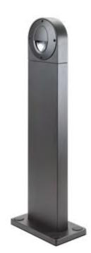
Small bollard with integrated LED chip, dimmable via phase cut dimming. Made from extruded and die-cast powder-coated aluminium, and glass diffuser. Class II means that it can be mounted without earthing, direct 230 V with loopable quick clips. 10-year corrosion warranty
