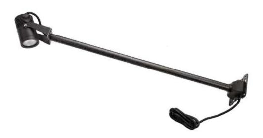
Hovden Sign is a signlight for outdoor use featuring a flexible luminaire head that can be turned towards wherever light is needed. Manufactured from powder-coated aluminium and supplied with a 10-year corrosion warranty. Supplied with a 1 meter cable with free end. Dimmable using phase cut. It includes an integrated, sealed light source which means the fixture is IP67 waterproof. Additional glare covers are available as accessories.
