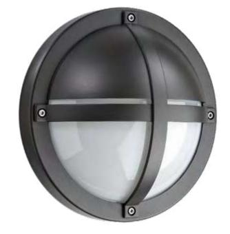
Attractive, round wall luminaire with half-diffuser and cross that can be installed both indoors and outdoors. Made of diecast powder-coated aluminium. Diffuser made of UV-stabilised opal polycarbonate. Two inputs/outputs for cables, option of both visible and concealed cabling, and loopable quick clips. Several variants with integrated sensor or dimming relay. Design: Hallvard Jakobsen
