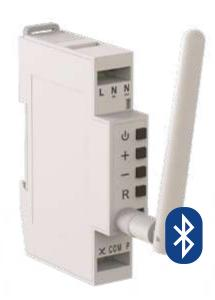
Bluetooth-controlled digital phase control dimmer for installation on DIN rail. Adjustable aerial to ensure good Bluetooth connection. Potential for control using pulse switch, either 230V or 24V.
