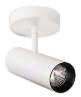
Slim, precise spotlight with a minimalist, exclusive look. Perfect for both ceiling and walls. Made of powder-coated, diecast aluminium and available in black or white finish. The retracted light source causes minimal glare and can be dimmed with trailing edge dimmer. Can be mounted on most known wall/ceiling electrical boxes.
