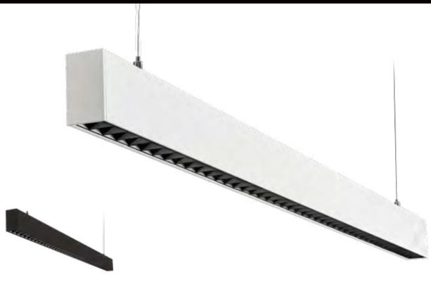
Ultra modern, slimline luminaires with powder-coated white outer surface. The cubist black reflectors provide extremely good glare control in direct light. Additionally, it features indirect light which means it is perfectly suited for offices and above desks. If you want to position several luminaires in a row, they can easily be connected together with the supplied coupling piece (no through wiring). Plug and play solution for quick installation.
