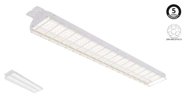
Arena Sport is an energy efficient surface mounted IP23 lumninaire for use in sports halls. It is easy to install with hinged gear tray, and can be mounted either direct on ceiling (screws) or suspended by wire. Arena Sport is available as single and double versions with two light distributions and protective grid. Available with DALI.
