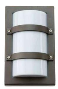
Square wall luminaire for extra protection of diffuser. Made of die-cast powder-coated aluminium. Diffuser made of UV-stabilised opal polycarbonate. Two inputs/outputs for cables, option of both visible and concealed cabling, and loopable quick clips. Corrosion-proof with 10-year warranty, IP65 and vandal-resistant rating IK10.
