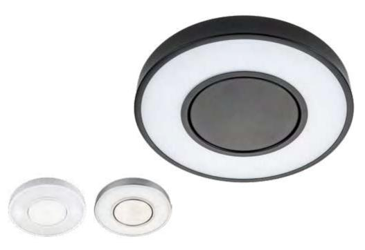
Round surface-mounted luminaire, wholly uniform light with attractive design, made of powder-coated steel, simple to mount by removing the back plate, which can be screwed on to all known ceiling outlets/ electrical boxes, clips with option of additional looping, connectors between lamp and mounting plate, dimmable driver phase cut/DALI and sensor options. Both visible and hidden cabling possible.
