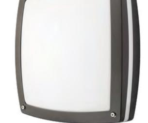
Attractive, square luminaire with direct and indirect light that can be mounted to both walls and ceilings, and both indoors and outdoors. Made of die-cast powder-coated aluminium. Flat diffuser with indirect light made of UV-stabilised opal polycarbonate. Design: Hallvard Jakobsen
